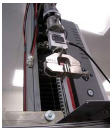
Adhesive testing (90° peeltest)
