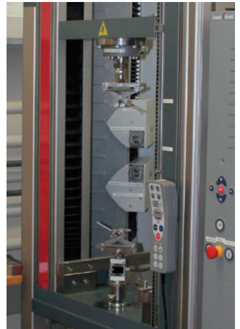
electro-mechanical test system
