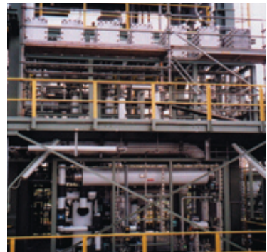
Seven modules in an industrial pervaporation plant
